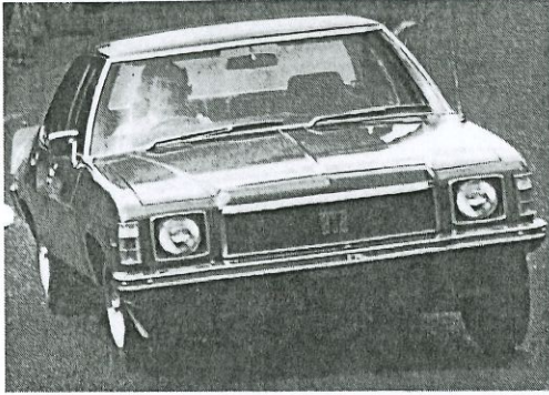
● THE Monaro GTS four-door combines the 4.2 litre V8 engine with the four-speed manual transmission as the standard power train.
